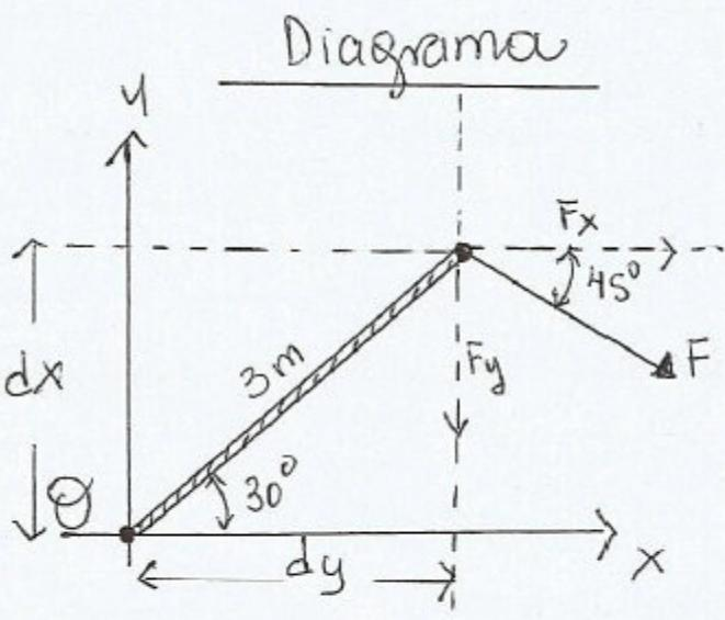
$$\Rightarrow M_{T\theta} = \underbrace{(F_x \parallel dx)}_{M_x} + \underbrace{(F_y \parallel dy)}_{M_y}$$
